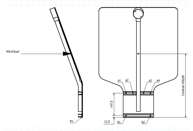
It is assumed that the wind loading is applied at the the centroid of the stucture. From this arrangement the loading and hence stresses in the rivets can be determined, assuming:
