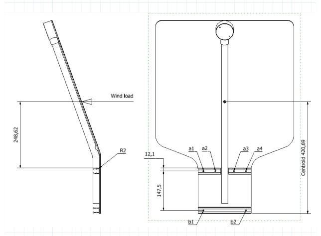
It is assumed that the wind loading is applied at the the centroid of the stucture. From this arrangement the loading and hence stresses in the rivets can be determined, assuming:
