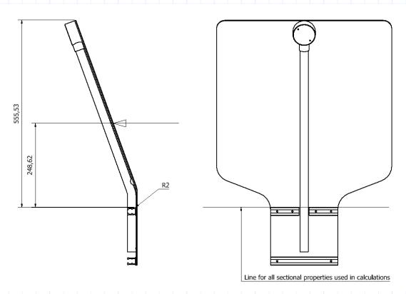
For calculation purposes the geometry of the assembly may be simplified to that in the following figure.
